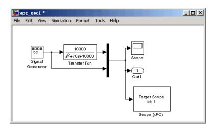
The model xpc\_osc1.mdl should look like the figure shown.
